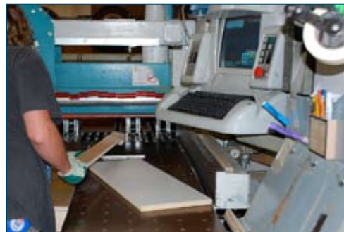
This computer driven saw allow us to get more from the same material, generating fewer wastes.
